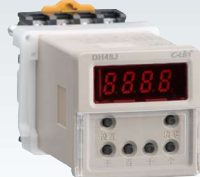
DH48J Counting relay Only for contact signal counting, if photoelectric switch/proximity switch counting is required, please choose the HHJ1 type
